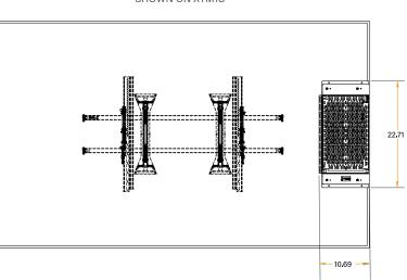
TYPICAL 86" DISPLAY 600MM MOUNTING PATTERN WIDTH SHOWN ON XTM1U
