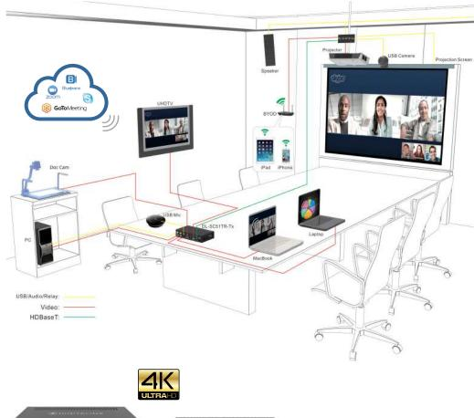
System automation built in! It automatically powers up TV or projector via RS232, up/ down relays for projector screens with no need for separate system control.
