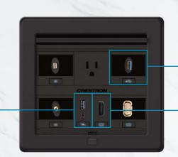
USB-A and USB-C can be used simultaneously Largest FlipTop option provides two separate connector bays facing opposite sides of the table
