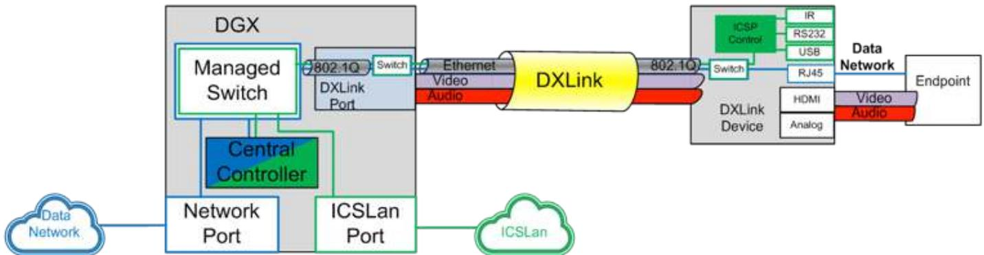
The Ethernet port on the DXLink device may be disabled, or assigned to either the ICSLAN or the enterprise network.
