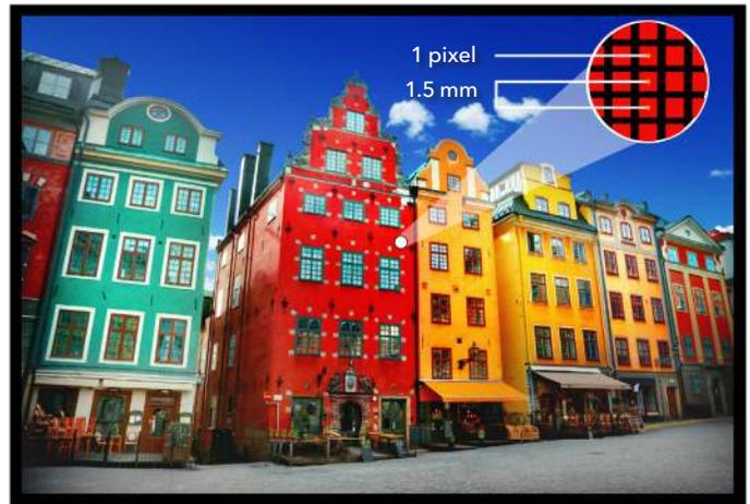
Image 5: Visual illustration of pixel pitch
